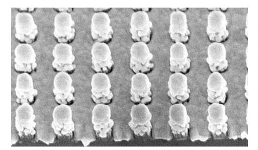
Princeton engineers have developed a sensor, seen in this micrograph, that gathers and amplifies Raman signals, which are wavelengths of light that can be used to identify substances. The sensor relies on a newly designed chip studded with uniform rows of tiny pillars made of metals and insulators. (Photo by Stephen Chou)
