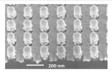
Micrograph of a sensor developed at Princeton for sensing Raman scattering. Pillars support metal components that gather light and amplify Raman signals, wavelengths of light that can be used to identify a substance.
