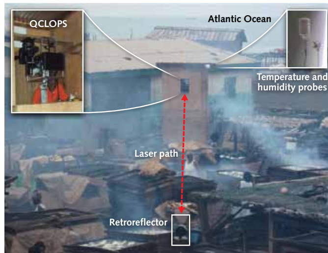
FIGURE 2. The MIRTHE QCL open-path system was deployed at Elmina, Ghana, on a day when many of the women were smoking fish. The picture shows the kiosk housing the sensor, the retroreflector, and the humidity sensor. The round-trip path length of the laser radiation is about 58 m. The signal from the detector is digitized and saved to a file using LabVIEW and alignment is aided with the help of a HeNe laser. (Image courtesy of MIRTHE)
